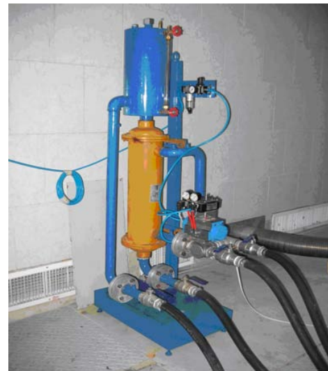
Fig. 2. Coolant conditioning system in engine test bed.
