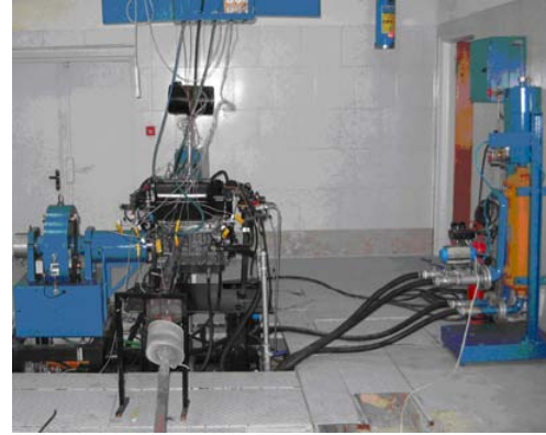
Fig. 1. Dynamometer, engine and coolant conditioning system.
